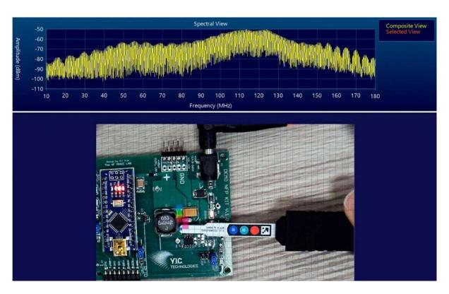
Live tracking provides a faster, easier, and more reliable method to get these results. Using an overhead webcam and probe markers, the EMViewer software will detect the type of probe and point of measurement automatically, allowing design engineers to see results quickly with minimal setup time.
