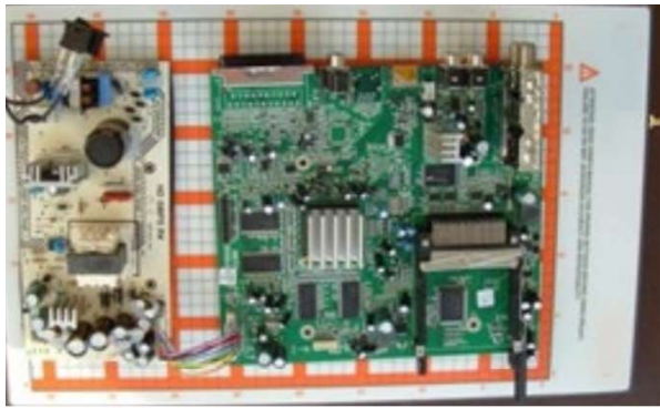
EMScanner spatial scan at 50MHz with no noise injection.
