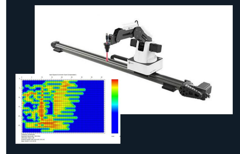
Single probe, articulated robotic arm Connect to Spectrum Analyzer and PC Runs EMViewer software Delivers repeatable and reliable results Design changes immediate EMProb diagnostics capabilities reduces testing time
