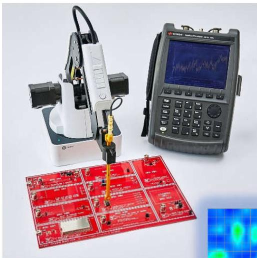
EMC and signal integrity are major concerns in the design of ultra-high speed (>2 GHz) PCBs. While EMScanner allows designers to easily locate emission by placing the PCB on its flat surface, the EMProbe allows users to test the component side of the PCB and adjust the height of the scan.
